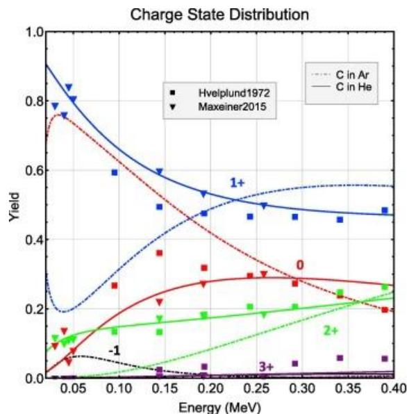
Charge state distribution of  $^{12}\text{C}$  with He and Ar stripping gases below 400 keV. Figure extracted from [2].
