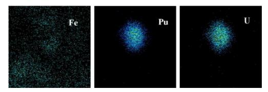
Elemental maps of Fe, Pu and U for a hot particle. The scan extent is  $75 \times 75 \mu m^2$ . Figure extracted from [3].
