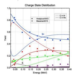
Charge state distribution of 12C with He and Ar stripping gases below 400 keV. Figure extracted from [2].
